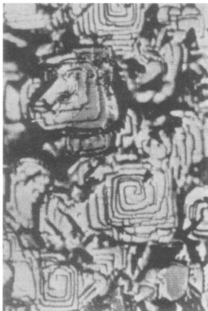
Figure 5.23 Spiral-formed growth [17] of a copper crystallite. Magnification 450 \times .
