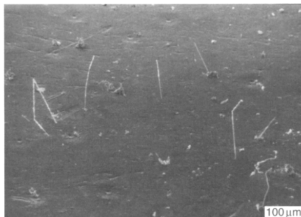
Figure 5.28 Whisker on the surface of zinc-plated steel cabinet (after 2 years in service).
